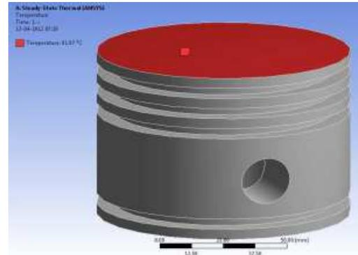
**Fig.3 Thermal boundary condition for Piston Head**
