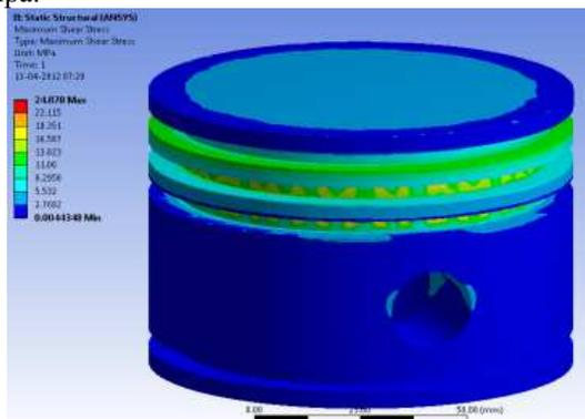
**Fig. 7 Shear Stress Distribution**
