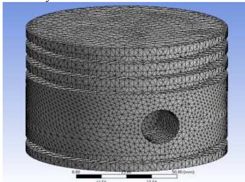
**Fig.2 Meshing in ANSYS of the Piston**
