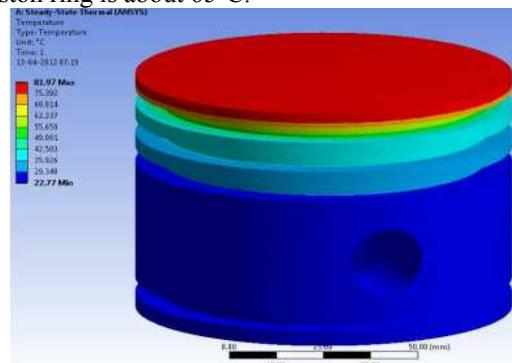
**Fig. 5 Temperature Profile Distribution of the Piston.**
