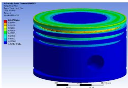
**Fig. 6 Total Heat Flux Transfer**
