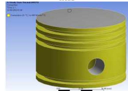
**Fig.4 Thermal Boundary Condition for Piston Length**
