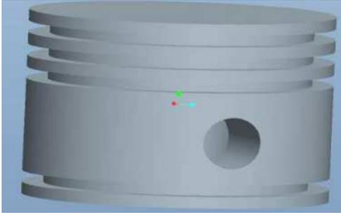
**Fig.1 Piston solid model generated by Creo-Elements**
