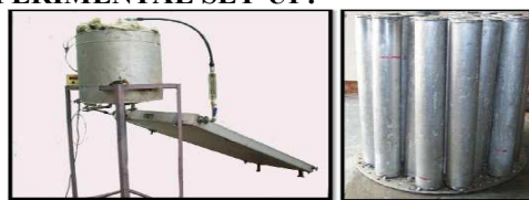
Figure 2: Experimental set up Figure 3: Aluminum tubes filled with PCM
