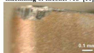
Fig.5. Flank wear during machining of Inconel 718 ( V_c=60 m/min, f=0.07 mm/rev)
