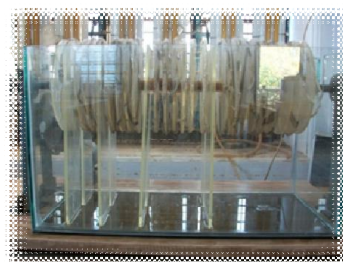
Figure 1: Lab-scale Rotating Biological Contactor
