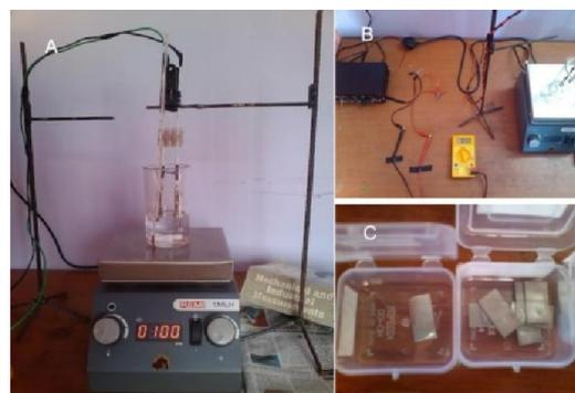
**Figure 1. (A) Electrochemical anodizing method Equipments setup in the Lab. (B) DC regulator (C) Titanium foil samples.**
