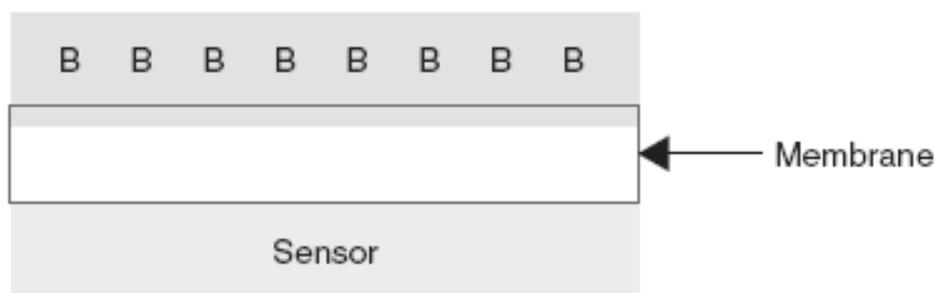
**Fig. 12 Physical Adsorption [6]**
