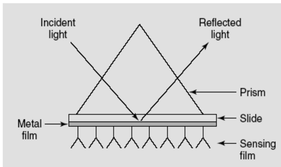
**Fig. 7 Kretschmann prism-based SPR Sensor [1]**
