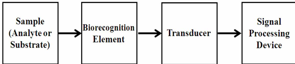
**Fig. 1 General scheme Of Biosensing [2]**
