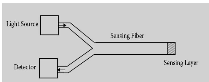
**Fig. 6 Configuration of Bio-Optrode [23]**
