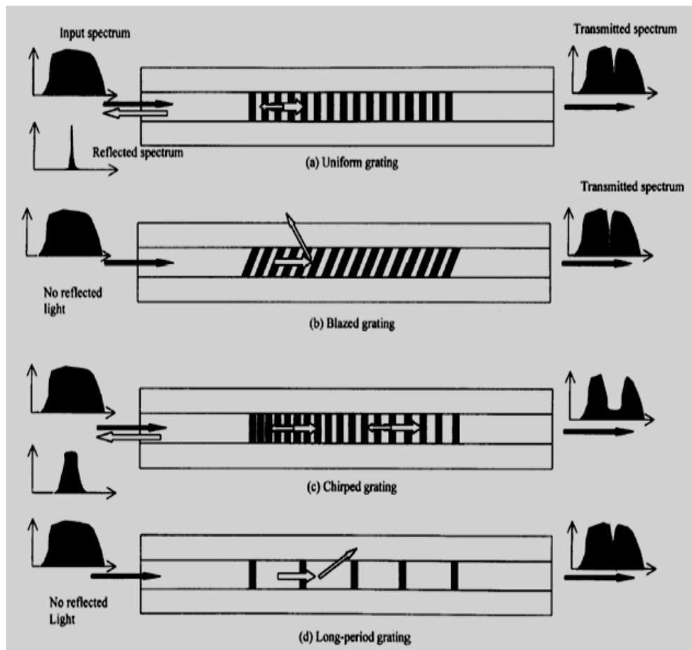
**Fig. 8 Different Types of Fiber Gratings [37]**
