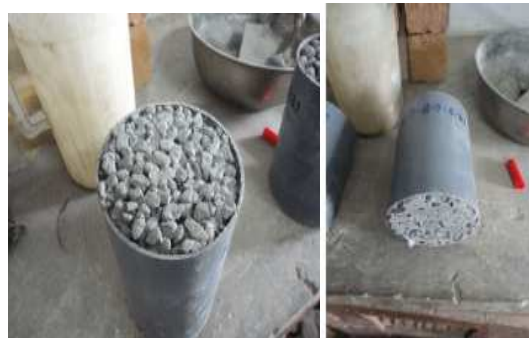
Figure 3a and 3b: Sample of Pervious concrete prepared for determination of permeability of concrete. Sample 1b (Mix: A-12.5-4.0-0.39), accumulation of paste at bottom of the specimen is visible which affect the permeability values of the mix.
