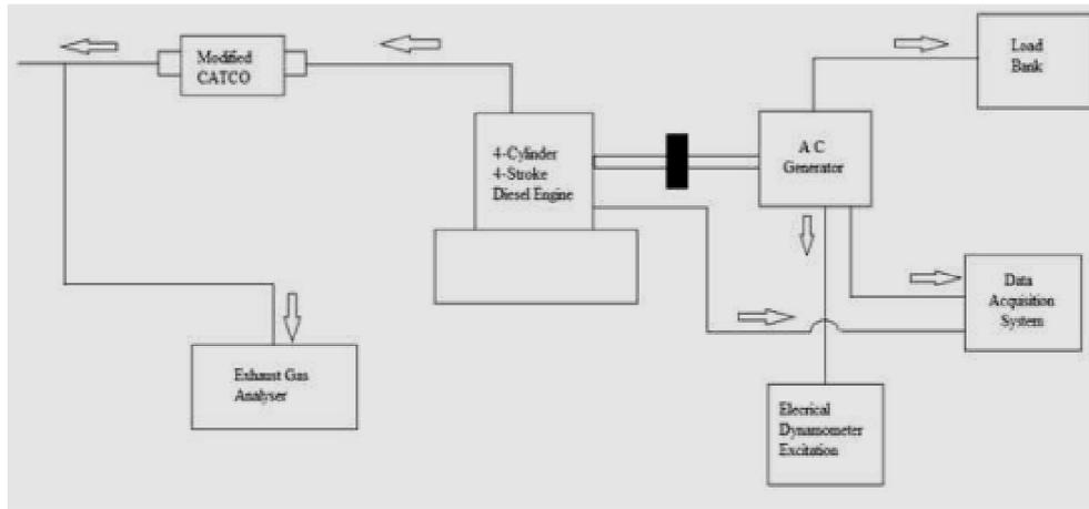
**Fig. 3 Layout of Experimental Setup**
