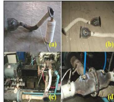
**Fig. 2 Various position of modified CATCO**
