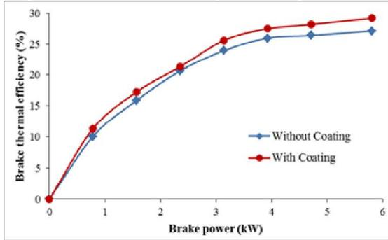
**Figure 1. Variation of brake thermal efficiency**
