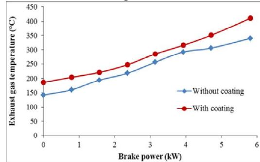
**Figure 3. Variation of exhaust gas temperature**
