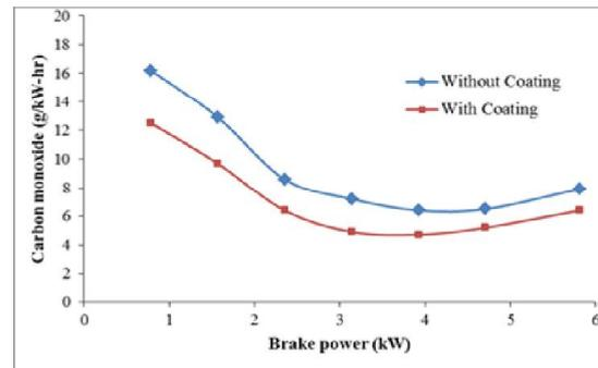
**Figure 4. Variation of carbon monoxide emission**
