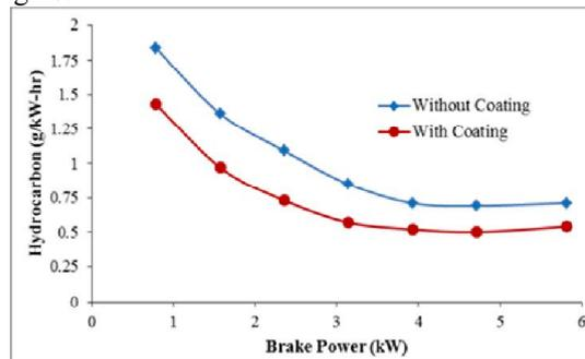
**Figure 5. Variation of unburned hydrocarbon emission**
