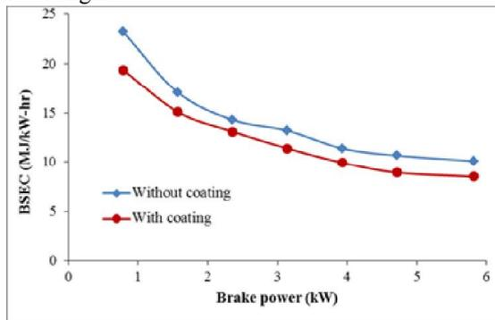
**Figure 2. Variation of brake specific energy consumption**
