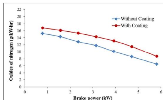
**Figure 6. Variation of oxides of nitrogen emission**
